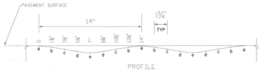
Figure 2. Sinusoidal Rumble Strip - Longitudinal Section
